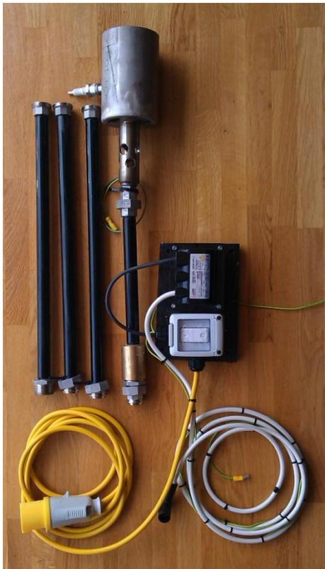
This flare conversion unit is designed for the direct venting of low pressure natural gas and LPG.
