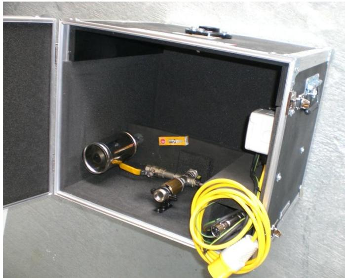
This purge unit is designed for the direct venting of natural gas and LPG up to 2bar. The flare burner unit also enables the unit to be used to burn off any gas where vented gas could cause a problem, due to smell etc. The single Flare Unit is similar to the large unit except that it has one burner and one ignition unit.
