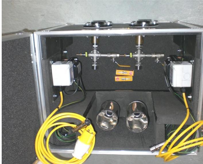
This Flare Unit is designed for the direct venting of natural gas and LPG. The flare burner can operate at pressures up to 2 bar and if necessary higher pressure supplies can be regulated to this pressure. The flare burner unit also enables the unit to be used to burn off any vented gas, where vented gas could cause a problem, due to smell etc. The twin Flare Unit is similar to the smaller unit except that it has two burners and two ignition units
