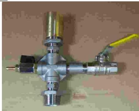
Attach one of the three 18" long 1/2" BSP steel uprights (with two unions) to the flame arrestor and valve assembly. Then screw it into the top steel flange of the main Purge Box using PTFE tape/sealant. Do not over tighten the joints.
