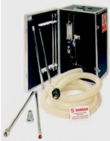
The purge unit is designed for the direct purging of pipework up to 150 mm bore from air to low pressure natural gas. It can also be used for natural gas to air purging but an air mover must be used which is available as an optional extra item. Larger Purge Units for above 150 mm bore pipework are also available. Please contact GEA for more information.
